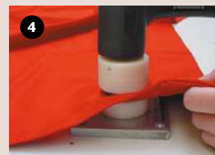
Rotate cutter top to ensure circle is cut all the way round.
