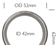
Metal Ring with Nylon Insert Ensures Quieter Running
