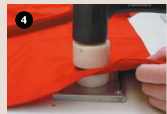
Rotate cutter top to ensure circle is cut all the way round.
