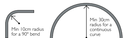
Mini-Optimal Track Bending Service: Single Angle Bend Code: 16OMBEND Continuous Curve Code: 16OMCONT
