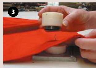
Align cutter top on the centre pin and then using a mallet, hit the cutter.
