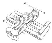
Slide blind slats in place and ensure to cut one slat at a time **ONLY**
