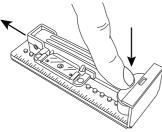
3 Lift up and then move the cutter left or right to adjust your trim length — use the metric or imperial gauge on the edges to assist you.
